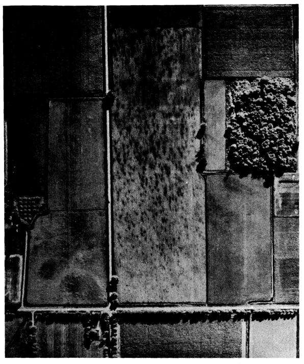
Figure 2. Enlarged black-and-white continuous tone separation from Kodak Ektachrome Infrared Aero film 8443 false color positive print. This reproduction shows only the red filter separation of the cyan dye layer. Dark foci in the center field indicate chlorophyll breakdown in bean plants affected by bacterial blight. Approximate scale: 1/2930,
